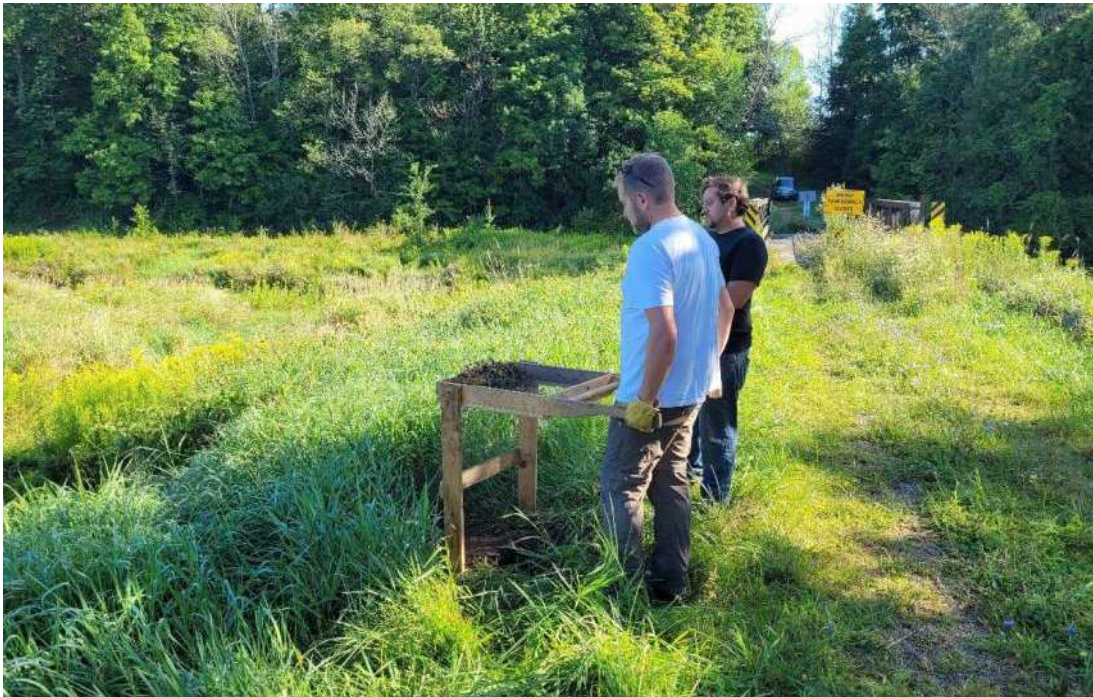
FIGURE 6: CONFIRMING FILL VIA TEST PITTING, FACING NORTH-NORTHEAST
